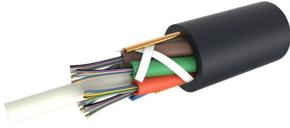
Fiber OSP cable, LightScope® ZWP Blown Micro Single Jacket All-Dielectric, Tone Wire Outdoor, 48 fiber, Stranded Loose Tube Arid-Core™ Construction, Gel-filled, Singlemode G.652.D and G.657.A1, Feet jacket marking, Black jacket color
