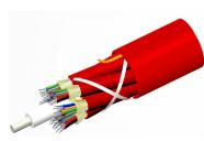
Fiber indoor cable, TeraSPEED® Plenum Distribution, 48 fiber multi-unit with 12 fiber subunits, Singlemode G.652.D and G.657.A1, Gel-free, Feet jacket marking, Red jacket color
