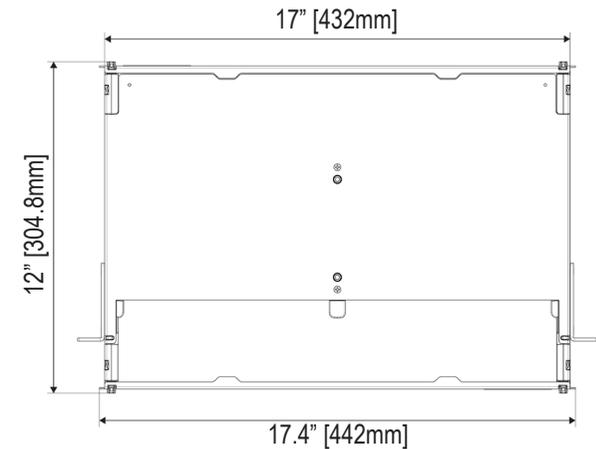
The overall width of the panels, including the mounting brackets, is 19" [482.6mm] or 23" [584.2mm] depending on which brackets are installed. The height of the panels can be found in this table:
