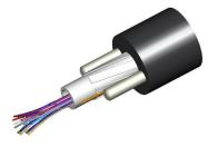
Fiber indoor/outdoor, TeraSPEED® Single Jacket Gel-Filled All-Dielectric Riser Rated Central Tube, 12 fibers, Singlemode G.652.D and G.657.A1, Feet jacket marking, black jacket color
