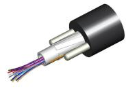
Fiber Indoor/Outdoor cable, Single Jacket Gel-Filled All-Dielectric Riser Rated Central Tube, 24 fibers, Singlemode G.657.A2/B2, Feet jacket marking, Black jacket color
