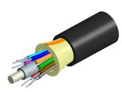
Fiber Indoor/Outdoor cable, TeraSPEED® Low Smoke Zero Halogen Riser Distribution, 18 fiber single-unit, Gel-free, Singlemode + Multimode OM4, Feet jacket marking, Black jacket color, Dca flame rating
