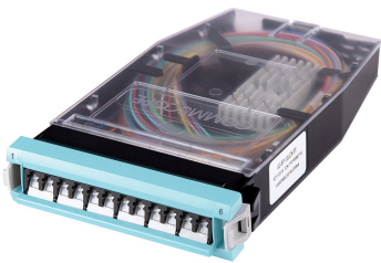
G2 Splice Cassette, 12LC with internal shutters, OM4, with 250um pigtails, Method B Enhanced
