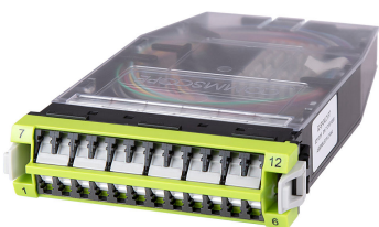
G2 Splice Cassette, 24LC with internal shutters, OM5, with 250um pigtails
