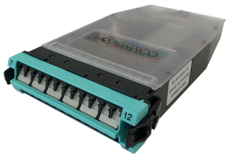
G2 Splice Cassette, 24LC with internal shutters, OM4, with 250um pigtails
