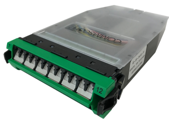
G2 Splice Cassette, 24LC/APC with internal shutters, OS2, with 250um pigtails
