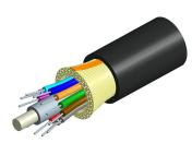
Fiber indoor/outdoor cable, LazrSPEED® Zero Halogen Riser Distribution, 2 fiber single-unit, Multimode OM3, Feet jacket marking, Black jacket color, Dca flame rating
