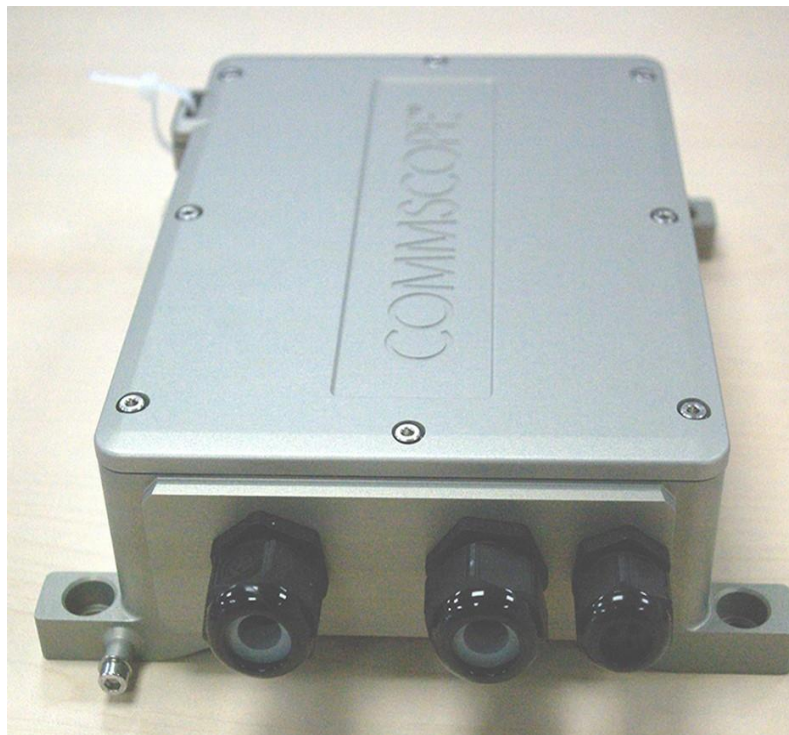
Figure 1: 2 Port 90 W PoE Extender (Heat Shield Removed)
