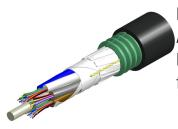
Fiber indoor/outdoor cable, TeraSPEED® Mini Single Jacket/Single Armor,Riser/LSZH rated, 8 fiber, Singlemode G.652.D and G.657.A1, Gel-Filled, Stranded Loose Tube, Black jacket color, Feet jacket marking, Dca flame rating
