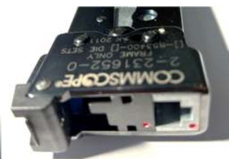
Hand crimp tool with pink dot crimp die
