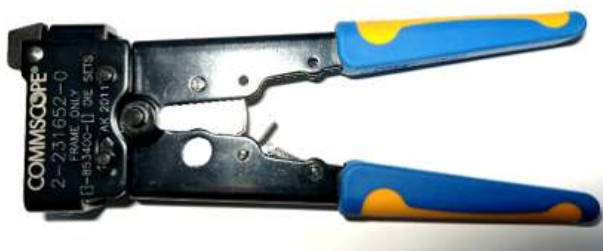
Hand crimp tool with pink dot crimp die
