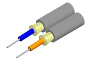
Fiber indoor cable, TeraSPEED® 2.9 mm Plenum Zipcord, Singlemode G. 652.D and G.657.A1, Feet jacket marking, Slate jacket color
