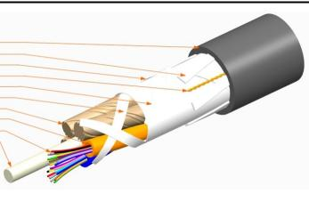
Plenum-Rated Outer Jacket Strength Elements Binder Water Swellable Tape Ripcord (1) Binder 2.5 mm Gel-Free Buffer Tubes 250 micron Fibers Dielectric Strength Member
