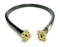
FlexTwist® Flexible Twist for WR62, 12.4–18.0 GHz, with interface types UG-419/U and UG-419/U, 300 mm
