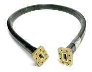
FlexTwist® Flexible Twist for WR62, 12.4–18.0 GHz, with interface types UG-419/U and UG-419/U, 900 mm
