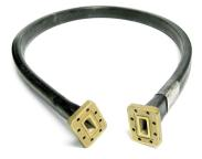
FlexTwist® Flexible Twist for WR62, 12.4–18.0 GHz, with interface types UG-419/U and UBR140, 600 mm
