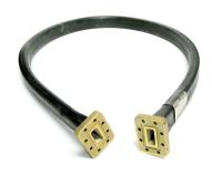
FlexTwist® Flexible Twist for WR90, 10.7–11.7 GHz, with interface types UG-39/U and CPR90G, 900 mm
