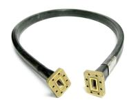
FlexTwist® Flexible Twist for WR90, 8.2–12.4 GHz, with interface types UDR100 and UBR100, 900 mm
