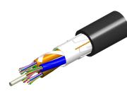
Fiber OSP cable, TeraSPEED® Light Duty, Single Jacket, 48 fiber, All-Dielectric, Gel-Free, Stranded Loose Tube, Singlemode G.652.D and G. 657.Al, Feet jacket marking, Black jacket color
