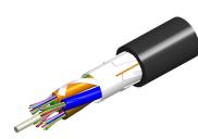
Fiber OSP cable, LazrSPEED®, Light Duty, Single Jacket, All-Dielectric, 36 fiber, Gel-Free, Stranded Loose Tube, Multimode OM4, Feet jacket marking, Black jacket color
