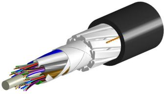
Fiber OSP cable, TeraSPEED® Mini Single Jacket All-Dielectric, High Tensile Strength, 36 fiber, Singlemode G.652.D and G.657.A1, Gel-Filled, Outdoor Stranded Loose Tube, Black jacket color, Feet cable marking, Provides Rodent Resistance
