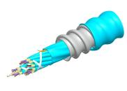
Fiber indoor cable, LazrSPEED® Riser/LSZH rated, MPO Trunk, interlocking aluminum armored, Multimode OM4, 36 fiber multi-unit with 12 fiber subunits, Gel-free, Feet jacket marking, Agua jacket color
