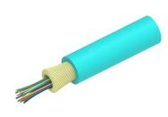
Fiber indoor cable, LazrSPEED® Plenum MPO Light Duty for Patchcords, 24 fiber, Multimode OM3, Feet jacket marking, Aqua jacket color
