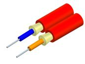
Fiber Indoor Cable, TeraSPEED® 1.6mm Low Smoke Zero Halogen Riser, 2-fiber Zipcord, Singlemode G.652.D and G.657.A1, Feet jacket marking, Red jacket color, Eca Flame Rating
