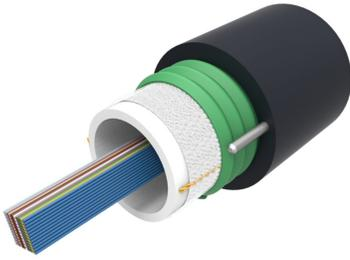
Fiber OSP cable, Steel Armored, Gel-Filled Central Tube Ribbon, 864 fiber, Singlemode G.652.D and G.657.A1, Feet jacket marking, Black jacket color
