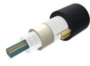
Fiber indoor/outdoor Cable, LSZH Riser All-Dielectric Central Tube Ribbon, Singlemode G.652.D and G.657.A1, 24-fiber, feet jacket marking, black jacket color
