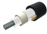
Fiber indoor/outdoor Cable, LSZH Riser All-Dielectric Central Tube Ribbon, Multimode OM3 bend insensitive, 12-fiber, feet jacket marking, black jacket color
