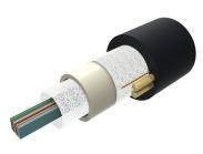
Fiber indoor/outdoor Cable, LSZH Riser All-Dielectric Central Tube Ribbon, Multimode OM4 bend insensitive, 48-fiber, feet jacket marking, black jacket color
