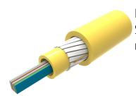
Fiber Indoor Cable, LSZH Riser, All-Dielectric, Central Tube Ribbon, Singlemode, G.652.D and G.657.Al, 12 Fibers, Gel-free, Feet jacket marking, Yellow jacket color
