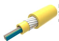
Fiber Indoor Cable, LSZH Riser, All-Dielectric, Central Tube Ribbon, Singlemode, G.652.D and G.657.Al, 24 Fibers, Gel-free, Feet jacket marking, Yellow jacket color
