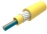
Fiber Indoor Cable, LSZH Riser, All-Dielectric, Central Tube Ribbon, Singlemode, G.652.D and G.657.A1, 24 Fibers, Gel-free, Feet jacket marking, Yellow jacket color
