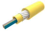
Fiber Indoor Cable, LSZH Riser, All-Dielectric, Central Tube Ribbon, Singlemode, G.652.D and G.657.A1, 36 Fibers, Gel-free, Feet jacket marking, Yellow jacket color
