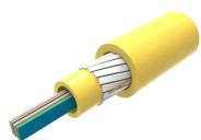
Fiber Indoor Cable, LSZH Riser, All-Dielectric, Central Tube Ribbon, Singlemode, G.652.D and G.657.Al, 72 Fibers, Gel-free, Feet jacket marking, Yellow jacket color
