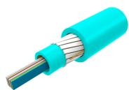
Fiber Indoor Cable, LSZH Riser, All-Dielectric, Central Tube Ribbon, Multimode, OM3, bend insensitive, 36 Fibers, Gel-free, Feet jacket marking, Aqua jacket color
