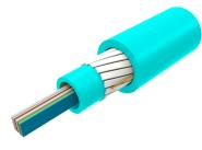
Fiber Indoor Cable, LSZH Riser, All-Dielectric, Central Tube Ribbon, Multimode, OM3, bend insensitive, 72 Fibers, Gel-free, Feet jacket marking, Aqua jacket color
