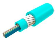
Fiber indoor cable, LSZH Riser All-Dielectric Central Tube Ribbon, 96 fiber, Multimode OM3 bend insensitive, Feet jacket marking, Aqua jacket color
