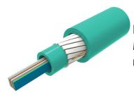
Fiber Indoor Cable, LSZH Riser, All-Dielectric, Central Tube Ribbon, Multimode, OM4, bend insensitive, 48 Fibers, Gel-free, Feet jacket marking, Aqua jacket color
