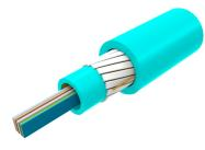
Fiber Indoor Cable, LSZH Riser, All-Dielectric, Central Tube Ribbon, Multimode, OM4, bend insensitive, 60 Fibers, Gel-free, Feet jacket marking, Aqua jacket color
