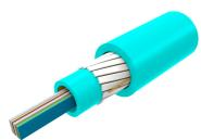
Fiber Indoor Cable, LSZH Riser, All-Dielectric, Central Tube Ribbon, Multimode, OM4, bend insensitive, 72 Fibers, Gel-free, Feet jacket marking, Aqua jacket color
