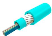
Fiber Indoor Cable, LSZH Riser, All-Dielectric, Central Tube Ribbon, Multimode, OM4, bend insensitive, 144 Fibers, Gel-free, Feet jacket marking, Agua jacket color
