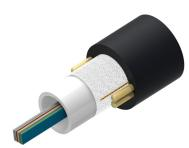
Fiber OSP Cable, Non-Armored, All-Dielectric, Gel-Filled Central Tube Ribbon, 36 fibers, Singlemode G.652.D and G.657.A1, Feet jacket marking, Black jacket color
