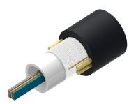
Fiber OSP Cable, Non-Armored, All-Dielectric, 864 fiber, Gel-Filled Central Tube Ribbon, Singlemode G.652.D and G.657.A1, Feet jacket marking, Black jacket color
