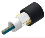
Fiber OSP Cable, Non-Armored, All-Dielectric, Gel-Filled Central Tube Ribbon, Multimode OM3 bend insensitive, Feet jacket marking, Black jacket color
