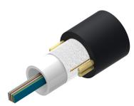
Fiber OSP Cable, Non-Armored, All-Dielectric, 192 fiber, Gel-Filled Central Tube Ribbon, Multimode OM3 bend insensitive, Feet jacket marking, Black jacket color
