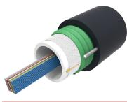
Fiber OSP cable, Steel Armored, Gel-Filled Central Tube Ribbon, 24 fiber, Multimode OM4, bend insensitive, Feet jacket marking, Black jacket color
