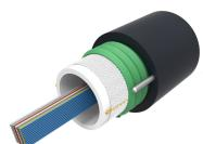
Fiber OSP cable, Steel Armored, Gel-Filled Central Tube Ribbon, 48 fiber, Multimode OM4, bend insensitive, Feet jacket marking, Black jacket color
