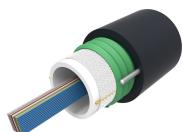
Fiber OSP cable, Steel Armored, Gel-Filled Central Tube Ribbon, 144 fiber, Multimode OM4, bend insensitive, Feet jacket marking, Black jacket color
